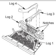
Figure 26 - Installing Logs 3 and 4
